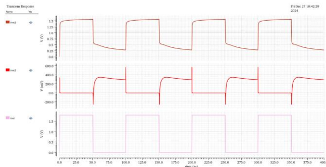
Figure 15. Output at each end of the inverter.
