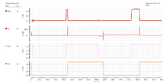
Figure 7. Output when the reference VCO is high.
